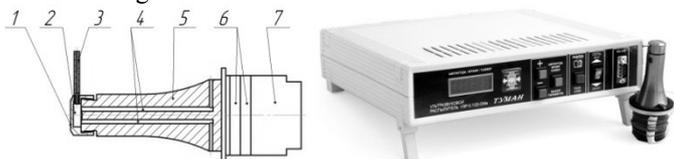
Fig. 7 – Ultrasonic atomizers of high-viscosity liquids
