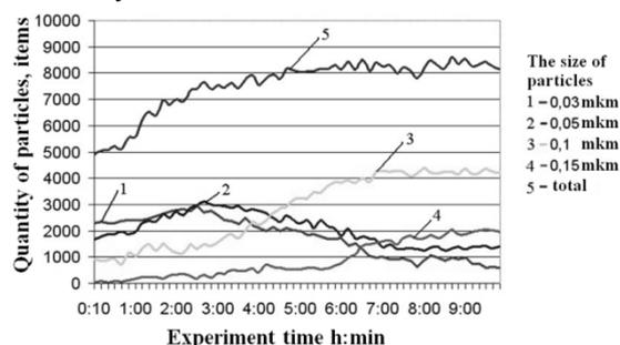
Fig. 6 – Dependence of quantity on the duration of ultrasonic influence and form of generated particles
