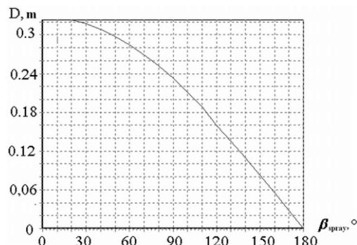
Fig. 3 – Dependence of diameter of torch of dispersion on spray corner
