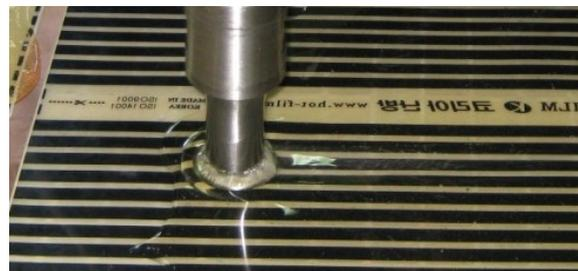
Fig. 5. The influence on the layer of epoxy resin deposited on the surface of the heating element.
