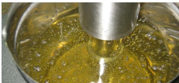
Fig. 3. The cavitation influence on epoxy resin.
