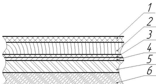
1 – linoleum, 2 – fibreboard or veneer wood, 3 – polyfilm, 4 – thermofilm, 5 – reflector-heat insulation, 6 – primary floor.
