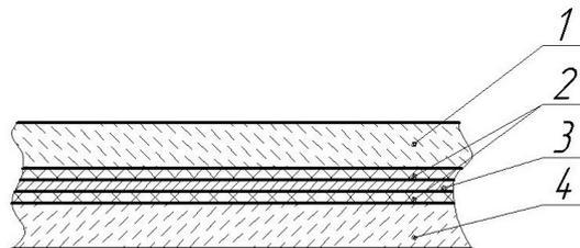
1 – stone flag with decorative or special coating, 2 – layer of epoxy resin, 3 – thermofilm, 4 – bearing stone flag
