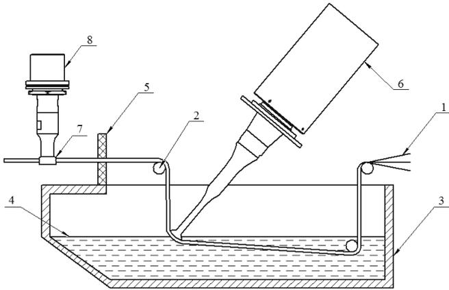
Fig. 4. The scheme of combined ultrasonic equipment for impregnation of polymer composite materials.
