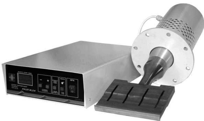
Fig. 1. The equipment for qualitative ultrasonic impregnation.
