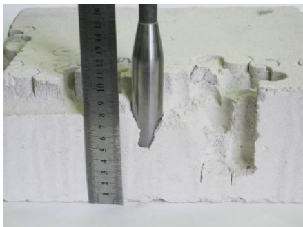
Fig. 11. The drilling process of foamed concrete block.
