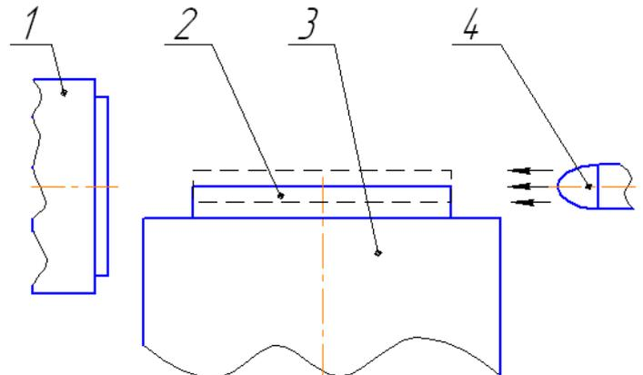
Fig. 4. The scheme of the bench for measuring of vibration amplitude, where 1 – the microscopic eyepiece, 2 – the end surface of the ultrasonic vibrating system, 3 – the technological volume with liquid, 4 – the stroboscopic lighting system
