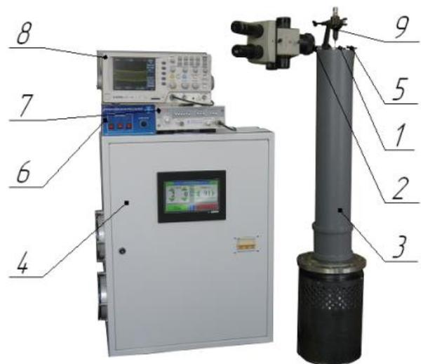
Fig. 5. The measuring bench, where 1 – the ultrasonic vibrating system, 2 – the microscope, 3 – the technological volume, 4 – the ultrasonic generator, 5 – the stroboscopic lighting system, 6 – the electronic impulse generator, 7 – the generator of model frequency, 8 – the oscillograph, 9 – sounding rod
