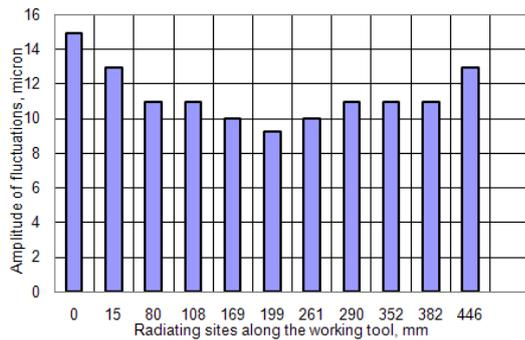
Fig. 6. The distribution of vibration amplitude of radiating surfaces of the tool along the axis
