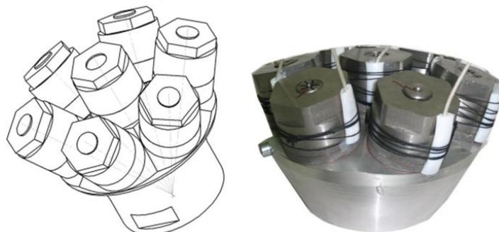
Fig. 2. The construction diagram of the multi-pack transducer
