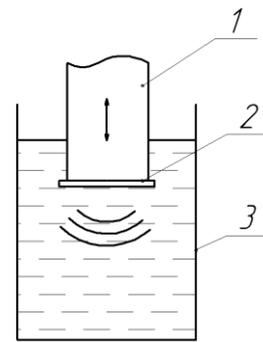
1 – wave-guide-concentrator; 2 – working tool; 3 – technological volume
