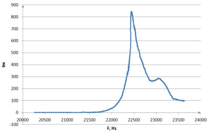
Fig. 4. Amplitude-frequency characteristic of the current of mechanical branch
