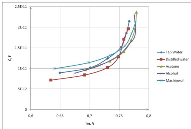
Fig. 8. The dependence of capacitance of the mechanical branch on the current of mechanical branch
