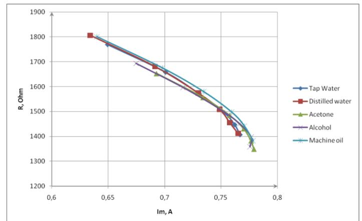
Fig. 6. The dependence of ohmic resistance of the mechanical branch on the current of the mechanical branch
