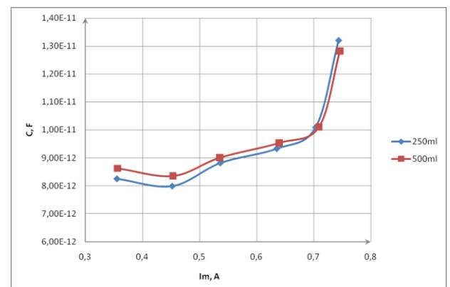
Fig. 11. The dependence of capacitance of the mechanical branch on the current of the mechanical branch
