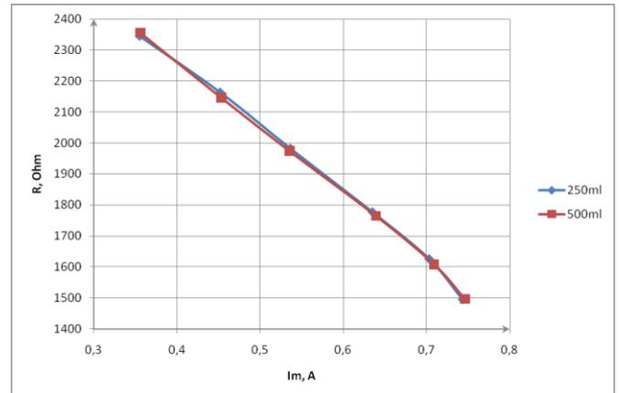
Fig. 9. The dependence of ohmic resistance of the mechanical branch on the current of the mechanical branch
