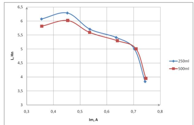
Fig. 10. The dependence of inductance of the mechanical branch on the current of the mechanical branch
