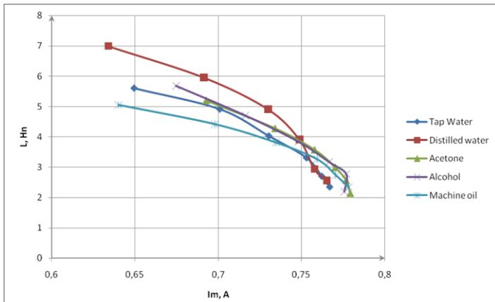
Fig. 7. The dependence of inductance of the mechanical branch on the current of the mechanical branch
