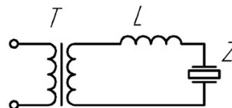
Fig. 1. The match circuit of the ultrasonic vibrating system with the output of the electronic generator
