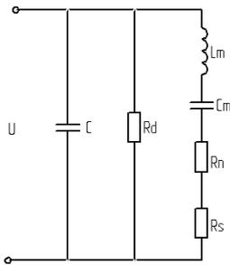
Fig. 2. The equivalent electric circuit of the ultrasonic vibrating system with the piezoelectric transducer
