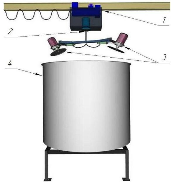
1 – transfer mechanism of the installation; 2 – electric motor; 3 – high-intensity radiators of ultrasonic vibrations; 4 – vessel
