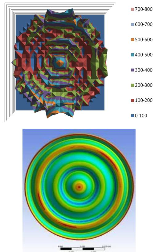
Fig. 3. The distribution of vibration amplitude on the surface of disk radiator Ø250 mm (on the left simulated, on the right measured)
