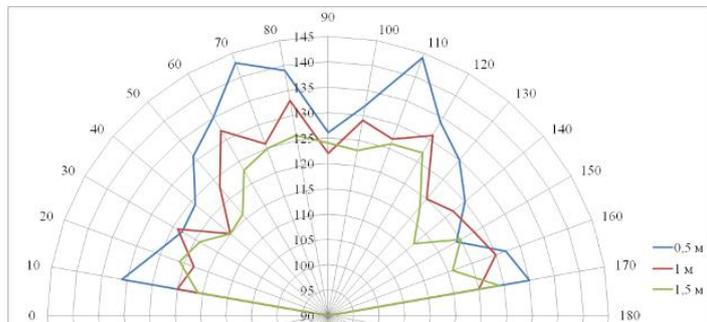
Figure 4 – The directivity pattern for the disk radiator Ø250 mm at the distance of 0.5 m; 1 m; 1.5 m without reflecting device
