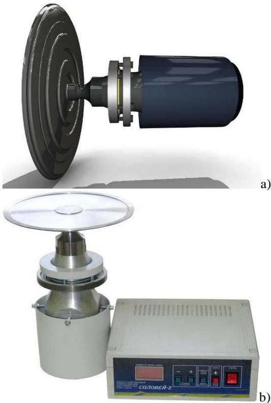
Fig. 1. 3-D model of the ultrasonic vibrating system with the radiator of the diameter of 250 mm (a) and the ultrasonic device with disk radiator of the diameter of 250 mm and the generator (b)
