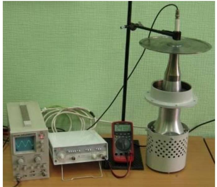
Fig. 2. The stand for measurements of distribution of vibration amplitude
