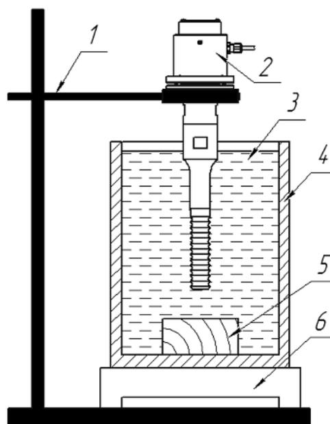
1 – stand, 2 – ultrasonic vibrating system, 3 – impregnating liquid, 4 – technological volume, 5 – sample to be impregnated, 6 – heating element
