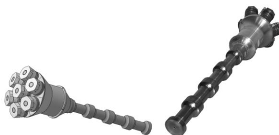
Fig. 2. Ultrasonic vibrating system with the multi half-wave radiator
