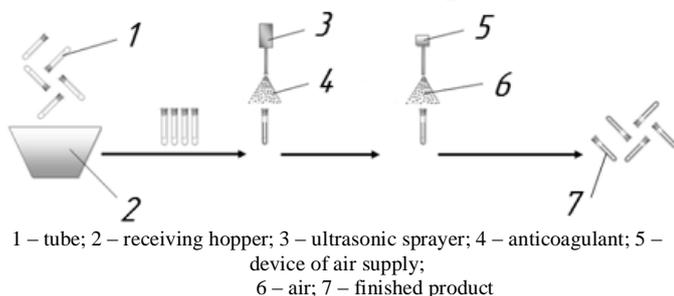
Fig. 1. Scheme of the ultrasonic spraying process of anticoagulant in the tube
