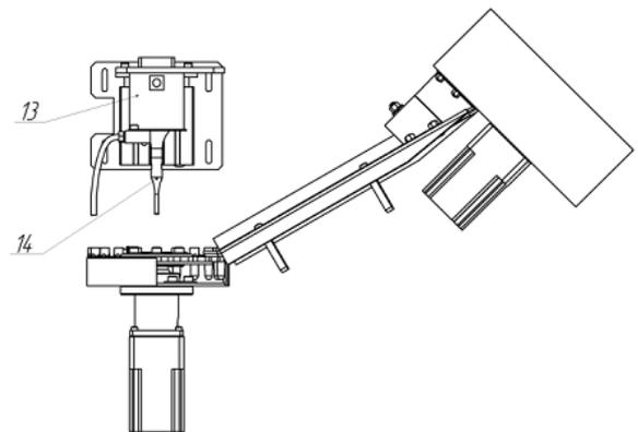
13 – piezoelectric transducer; 14 – horn
