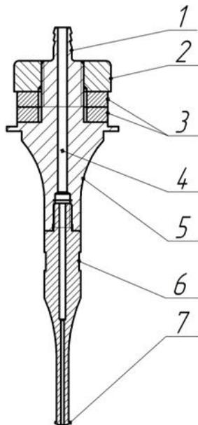
1 – fitting for fluid supply; 2 – reflecting plate; 3 – piezoelectric elements; 4 – channel for fluid supply; 5 – horn; 6 – horn-waveguide; 7 – spraying end
