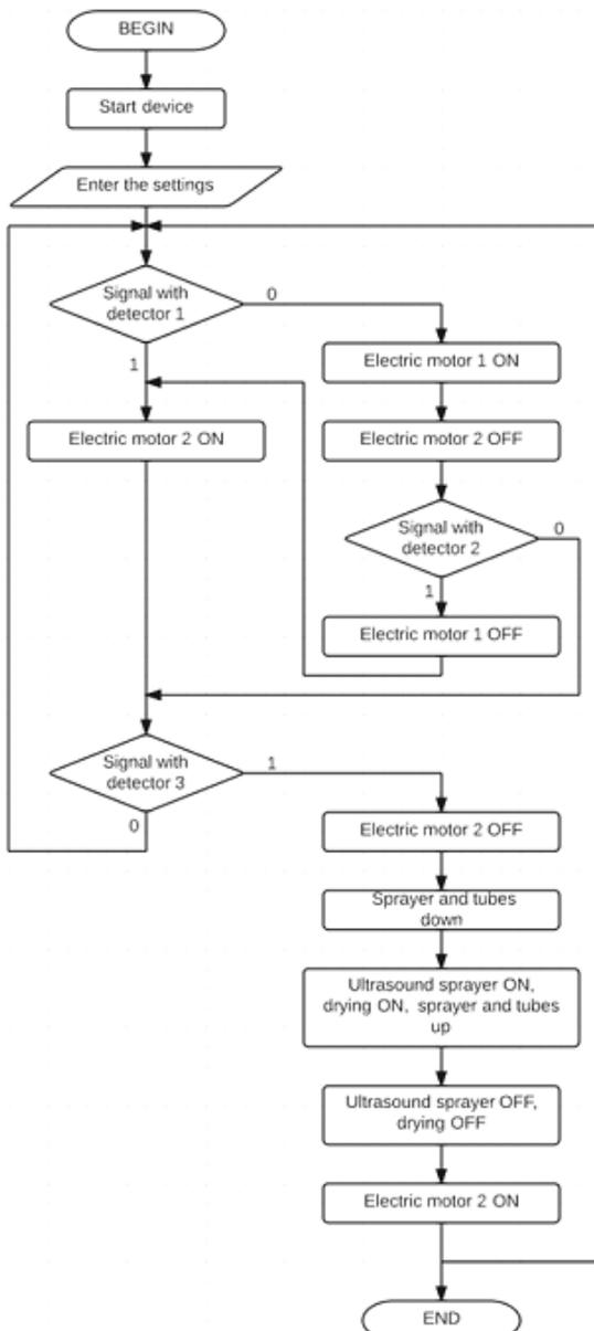
Fig. 6. Control algorithm of automated line operation
