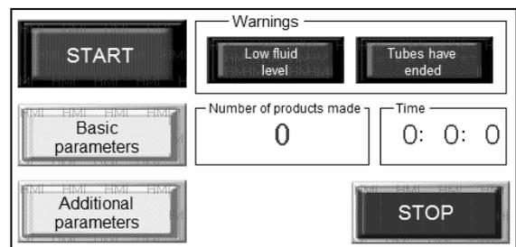
Fig. 7. Main working interface of the operator of the line
