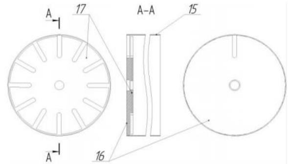
15 – hollow cylinder, 16 – fixed disc; 17 – movable disc
