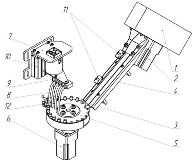
1 – hopper, a piece dispenser of the tubes; 2 – electric motor; 3 – tube; 4 – directing runners; 5 – disc for moving of the tubes; 6 – electric motor; 7 – sprayer; 8 – pipes for the supply of drying agent; 9 – footlights for supplying of drying agent; 10 – device of vertical movement; 11 – optical detector for the control of the tubes on directing runners; 12 – optical detector for the positioning of the disc
