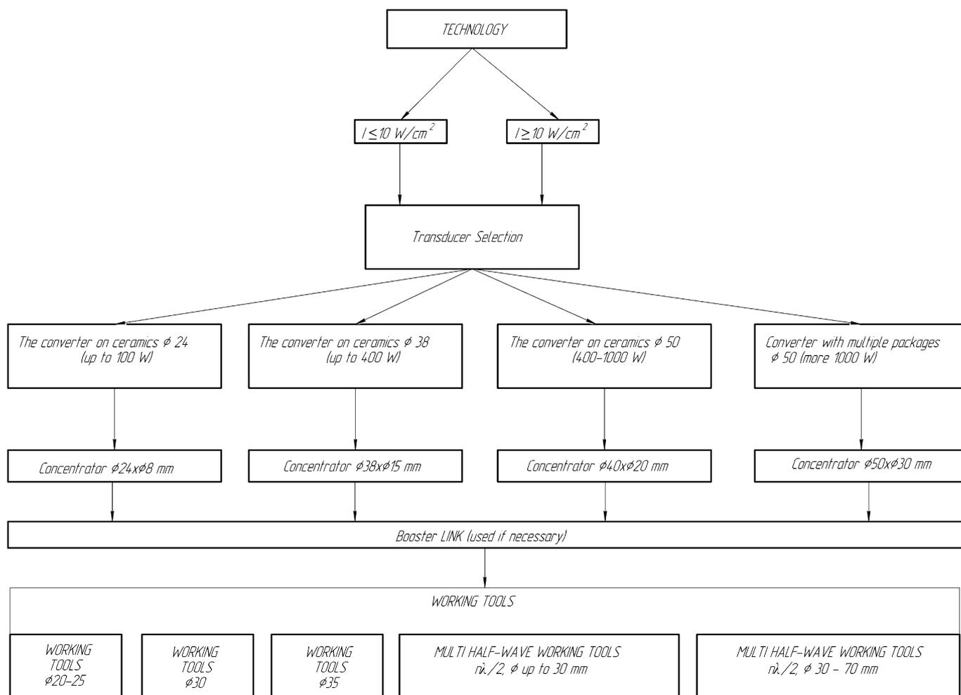
Fig. 1. Scheme of the choice of ultrasonic vibrating system
