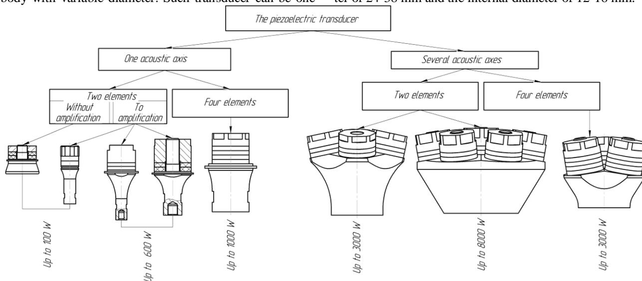
Fig. 2. Choice of the piezoelectric transducer
