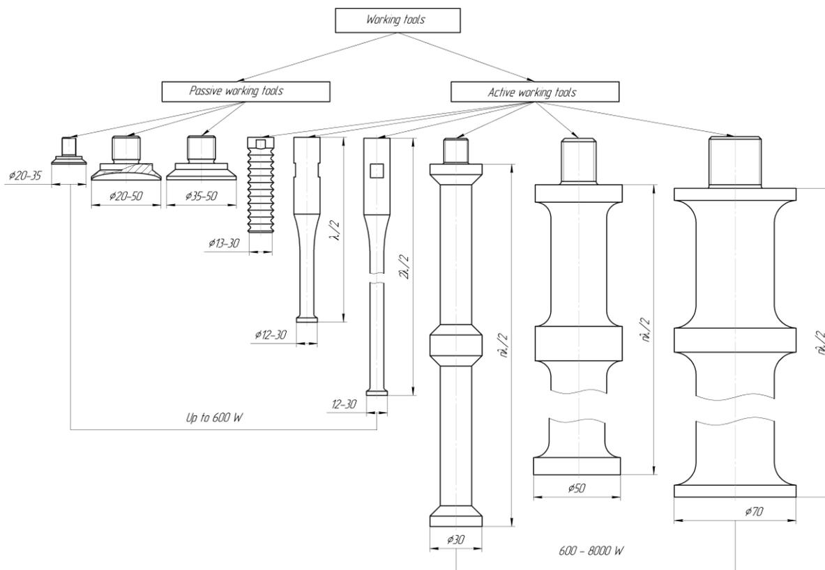
Fig. 4. Scheme of the choice of working tool
