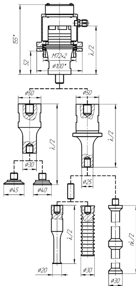
Fig. 5. Choice of the ultrasonic vibrating system by the step-by-step selection of single structural components
