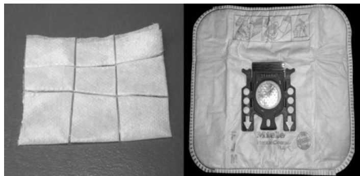
Fig. 1. Examples of formed seams and the articles with continuous welding seams.
