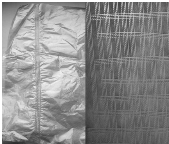
Fig. 9. Examples of welding seams made with the application of the ultrasonic equipment.
