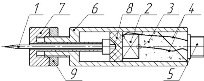
1 – metal waveguide; 2 – piezoelectric element; 3 – damper (epoxy compound); 4 – wires; 5 – electrical connector; 6 – case; 7 – cylindrical bushing with the screw nut; 8 – elastic layer made of sound-absorbing material; 9 – check-nut
