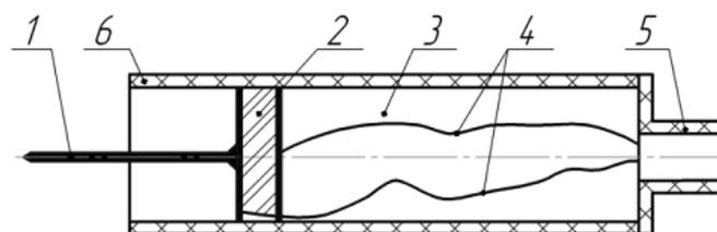
1 – metal rod; 2 – piezoelectric element; 3 – damper (epoxy compound); 4 – connecting wires; 5 – electrical connector; 6 – case.
