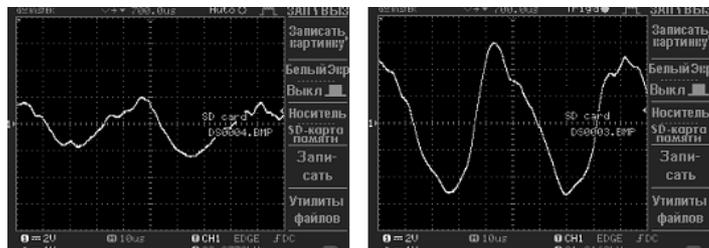
Fig. 3. Maximums and minimums of the vibration amplitude at the excess pressure.
