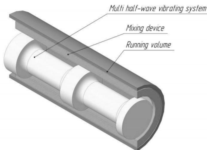
Fig. 7. Fragment of running volume with mixing device.
