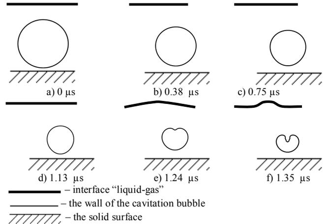
Fig. 2. Development of the form of asymmetrically collapsing cavitation bubble in the course of time.
