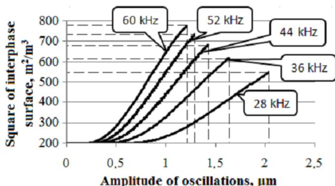
Fig. 3. Dependences of specific area of the interface on amplitude at different frequencies.
