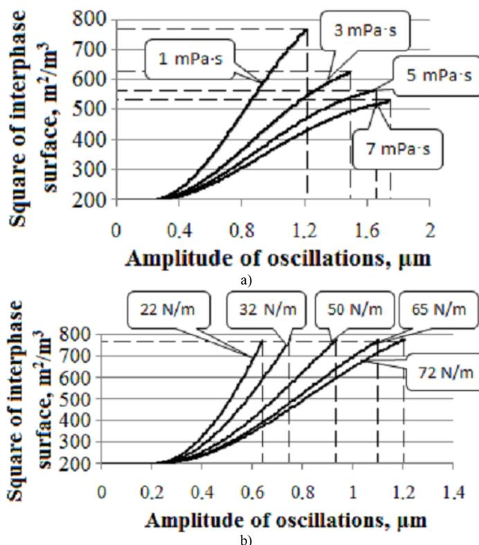
Fig. 4. Dependences of a square of the interphase boundary area on amplitude at various liquid properties (frequency of 60 kHz).
