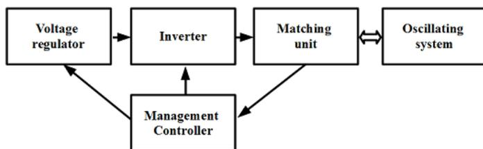
Fig. 1. Main block diagram of the ultrasonic generator
