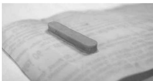
Fig. 7. Results of welding of firm polymer plate to the material of the pack.
